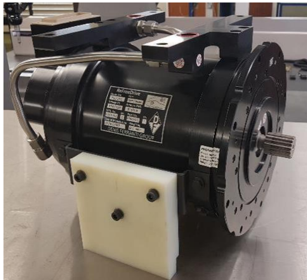
Figure 1 ReFreeDrive Induction Machine complete assembly.
