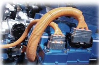
High voltage wiring
