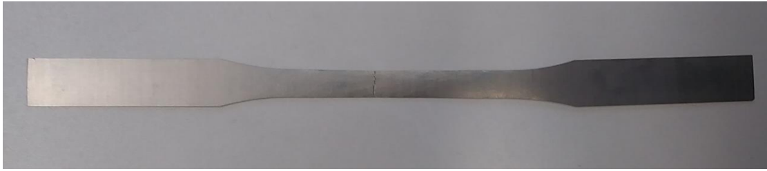
Figure 5. Electrical steel specimen after a tensile test
