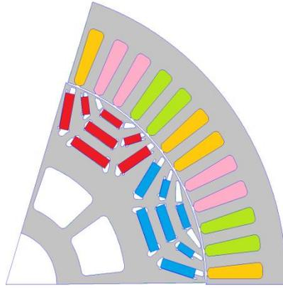
Fig. 8 PM assisted synchronous reluctance motor design
