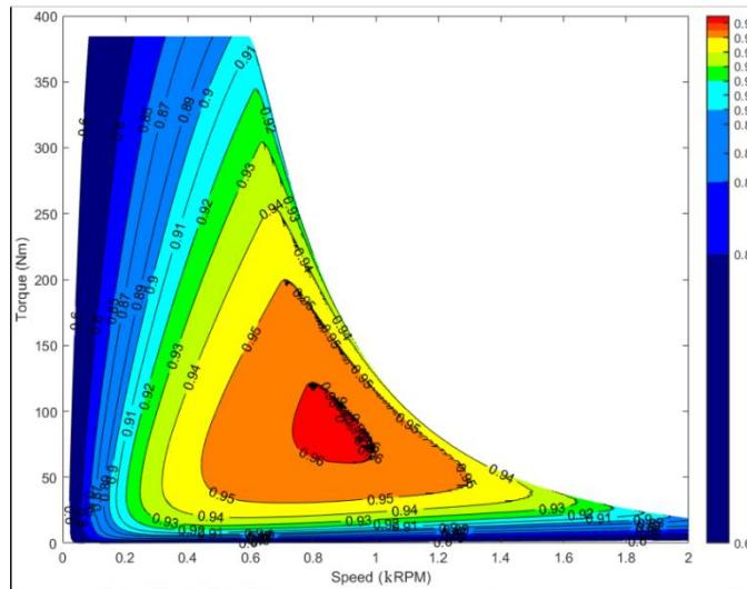
Fig. 7 200kW pure synchronous reluctance motor efficiency map
