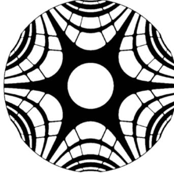
Fig. 6 Rotor shape of the 6-poles machine
