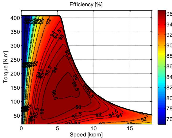
Fig. 9 200kW PM assisted synchronous reluctance motor efficiency map
