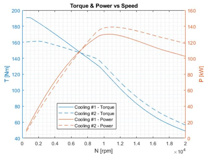
Fig. 5 Comparison between continuous performance of cooling system (1) and (2)
