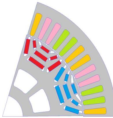
Fig. 8 PM assisted synchronous reluctance motor design
