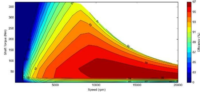
Fig. 4 Efficiency map for inner rotor CR-IM, with M235-35A steel
