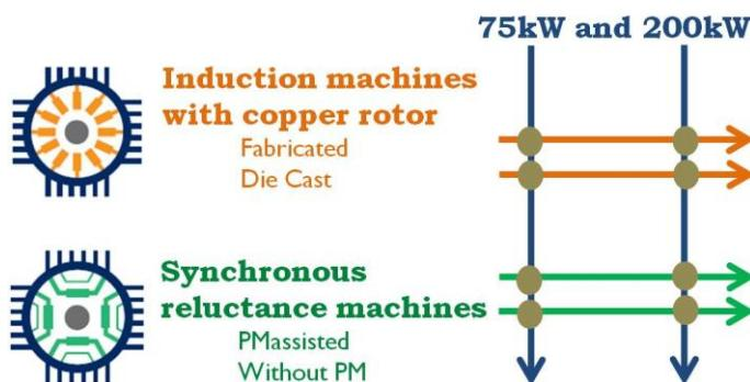
Fig. 2 Motor technologies and use cases considered in ReFreeDrive project
