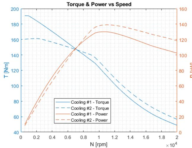
Fig. 5 Comparison between continuous performance of cooling system (1) and (2)
