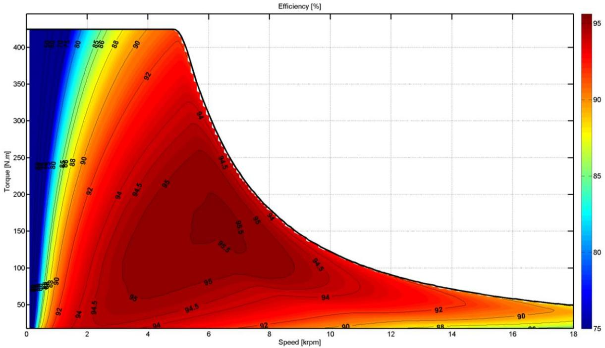
Figure 6: Torque vs Speed efficiency map of 200kW PMA-SynRel Motor
