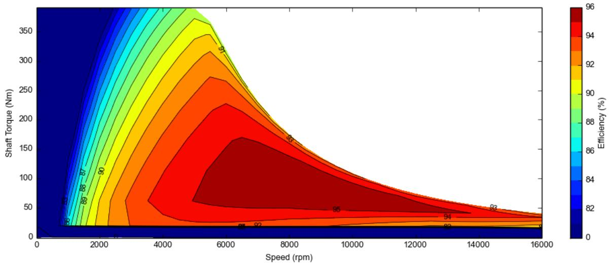
Figure 7: Torque vs Speed efficiency map of 200kW pure SynRel Motor
