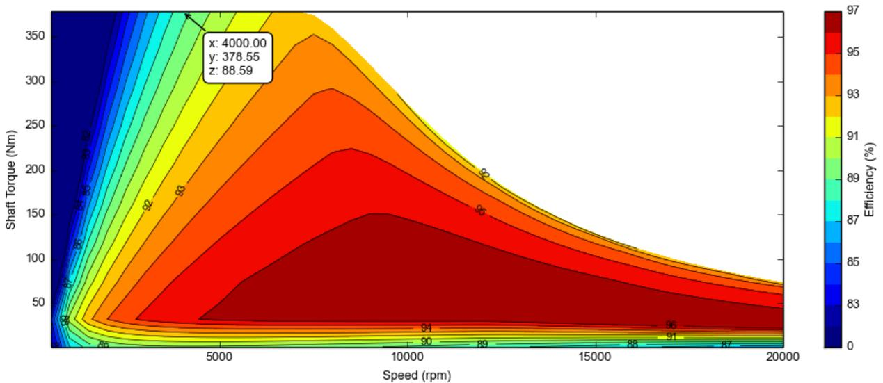
Figure 4: Torque vs Speed efficiency map of 200kW IM
