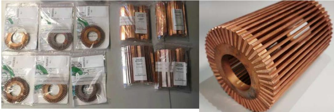
Figure 58: Induction motor fabricated copper cage (assembled for demonstration purposes).
