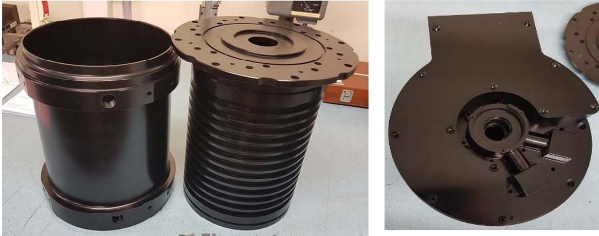
Figure 11: Cooling Jacket manufactured in Aluminium, for Induction machines
