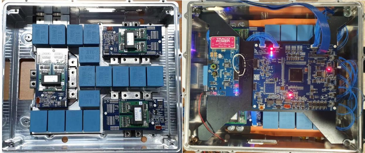
**Figure 20: Different layers of 75kW REFREEDRIVE power electronic prototype, on housing, taken from D6.9**
