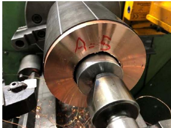
Figure 57: End-ring at melt ingate side, after machining.
