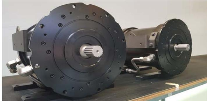
**Figure 59: Induction Machine complete assembly**
