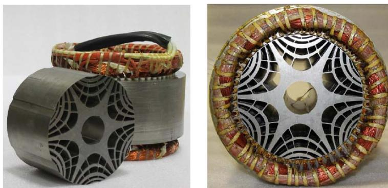
Figure 5: Wound stator and rotor core for a 75 kW Pure SynRel motor (Deliverable 6.3)
