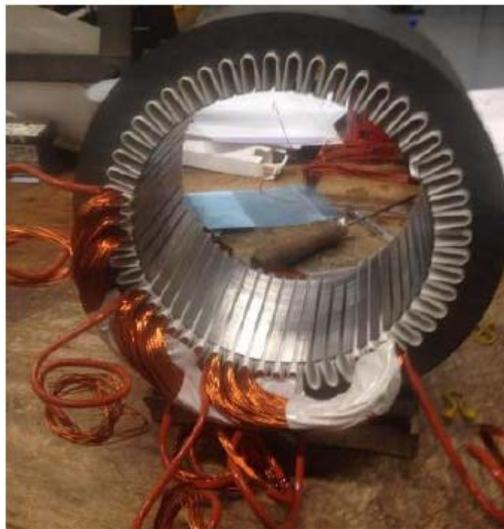
**Figure 44: Manufacturing processes of the 75 kW stator winding**
