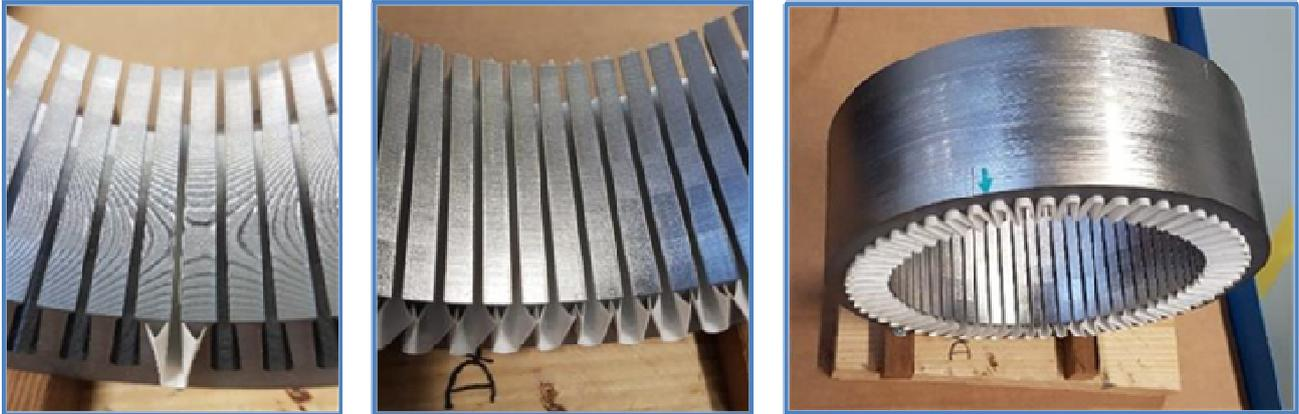
Figure 34: Slot liner insertion into the stator slots for a PMa SynRel motor (Deliverable 6.4)
