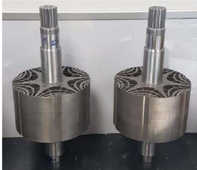
Figure 46: Insertion of rotor stacks on shaft
