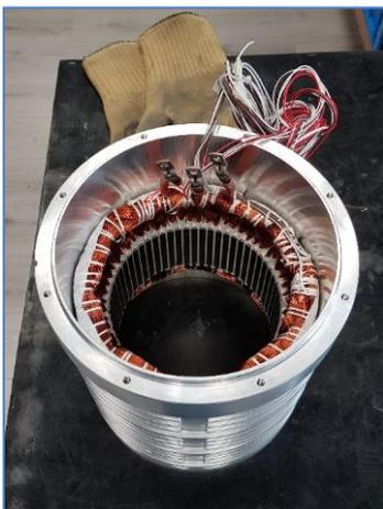
Figure 40: Stator insertion in the cooling jacket
