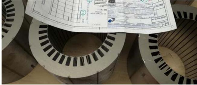
Figure 50: Stator stacks for the IMs (each stator is built with 36 slots).
