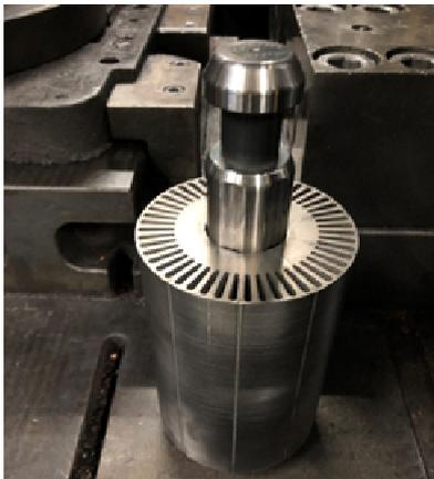
Figure 56: Stack on casting mandrel.
