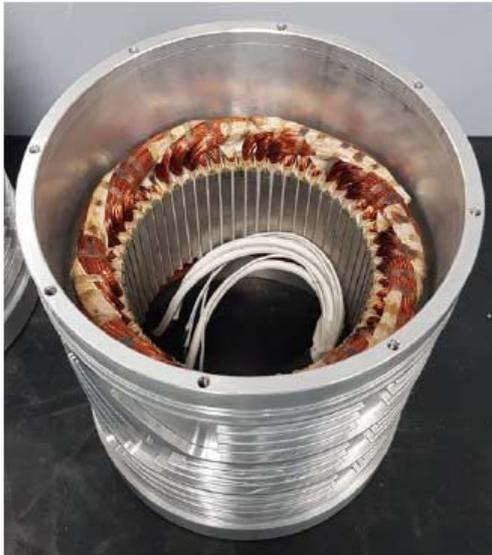
Figure 47: Wound stator insertion in the internal cooling case
