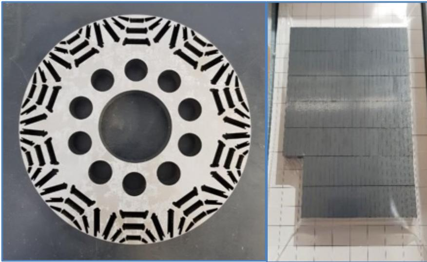
Figure 37: Rotor core, Permanent Magnets (PMs)
