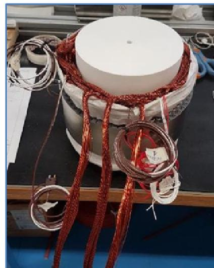
Figure 36: Wires separation, taping and coil forming
