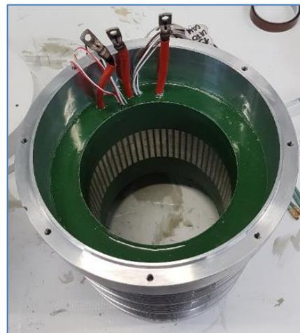
Figure 41: Stator potting final result
