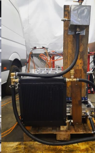
Fig. 13 The test bench with the CC of the BP, radiator, tank and pump
