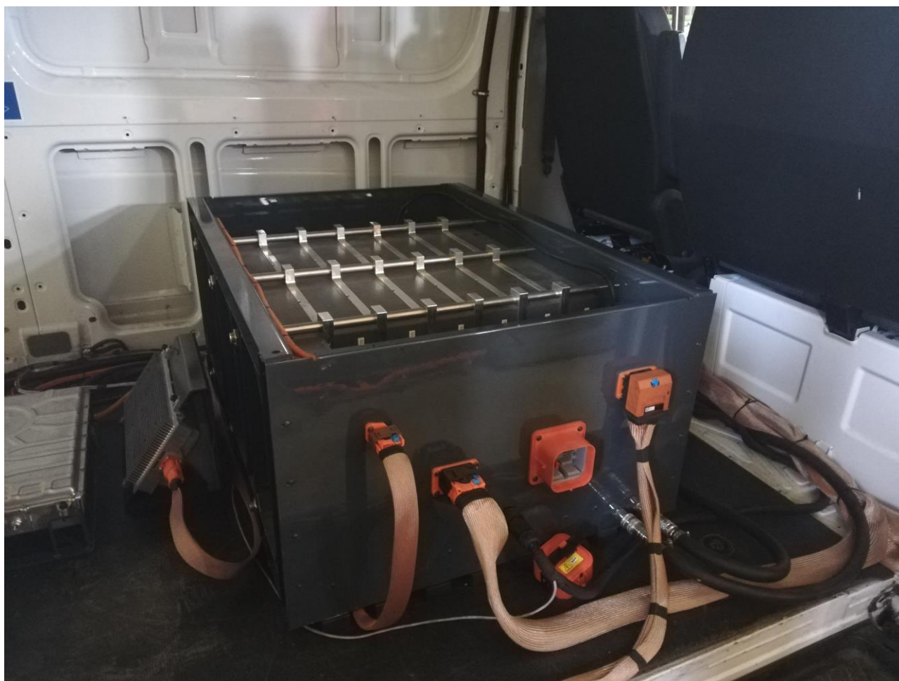
Fig.2 BP installed in the vehicle and HV routing
