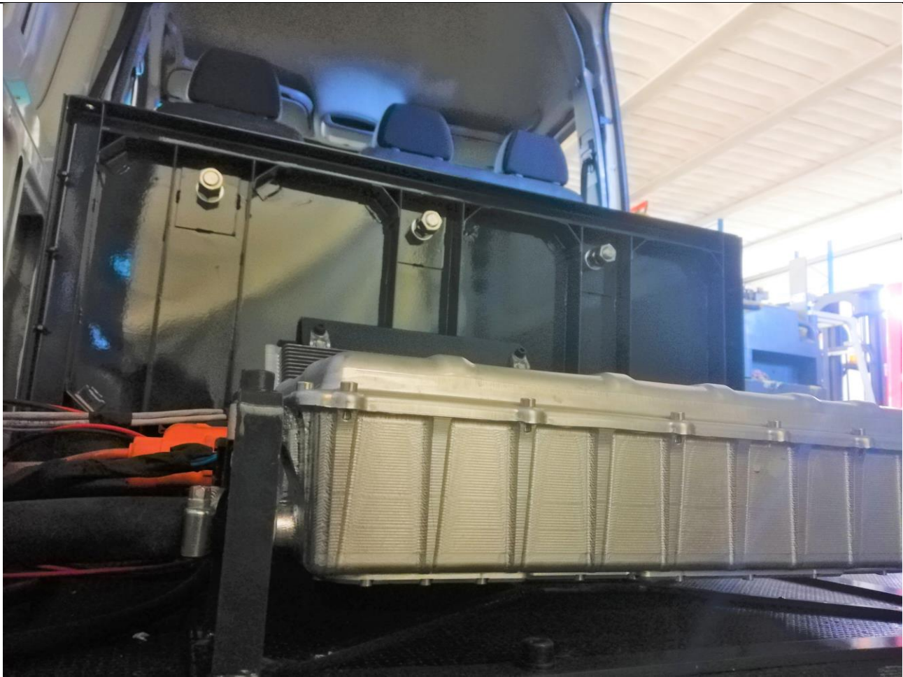
Fig. 7 Connection of the charger with the Sprinter chassis
