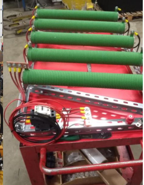
Fig. 14 The resistors test bench to test the discharge of the BP, 5 resistors of 2kw each and 100 Ohm
