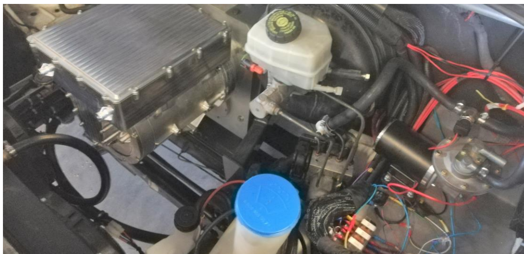
Fig. 10 View of the PB, PS and fuses box
