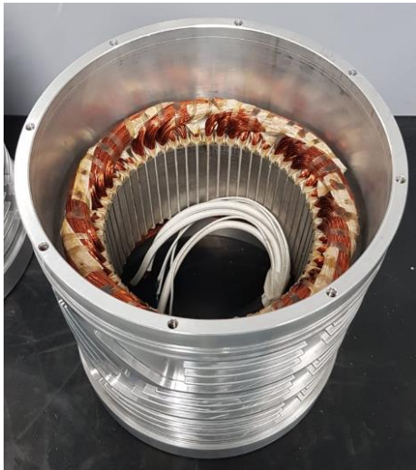
Figure 10: Wound stator insertion in the cooling jacket
