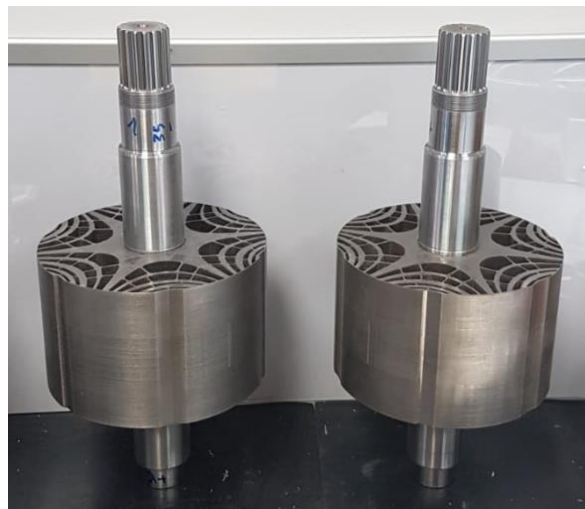
Figure 11: Insertion of rotor stacks on shaft
