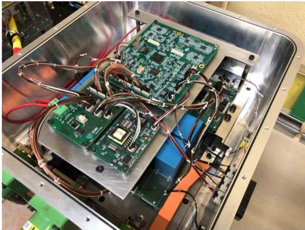
Figure 1: High Power Range 800V Power Electronics prototype (435kVA)
