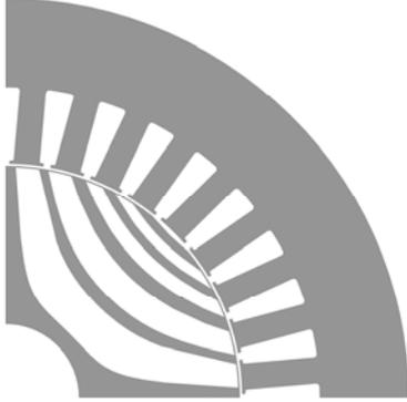
Fig. 2. Cross section of the optimal 4-poles design
