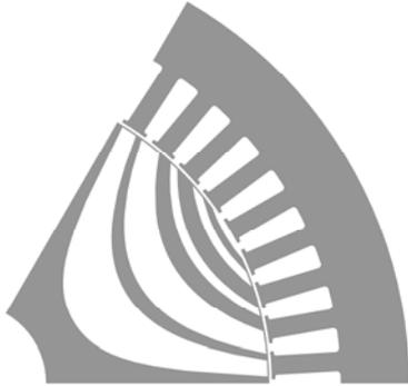
Fig. 3. Cross section of the 6-poles preliminary design
