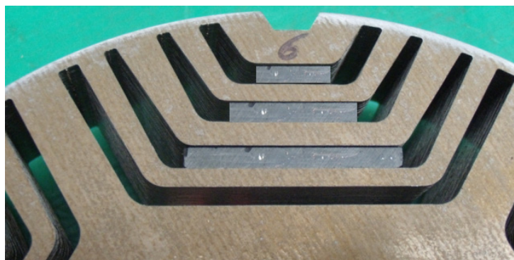
Fig.6 Rotor of PM-assisted synchronous reluctance motor (in Ferrite)
